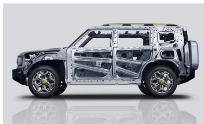
32000N/M/DEG BODY TORSIONAL STIFFNESS
