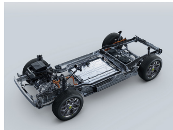
26.7KWH HIGH-CAPACITY BATTERY
